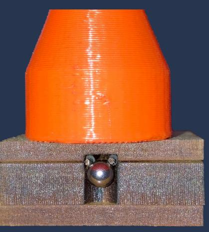
Magnet in player piece lifts steel ball inside the board to close a circuit, indicating player positions
